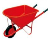
➤ WB0601P Load Capacity:10kg Water Capacity:21L Sand Capacity:1CBF Wheel:8" x1.75" Solid L/H/C/A/B/h(mm):852x320x292x590x432x218
