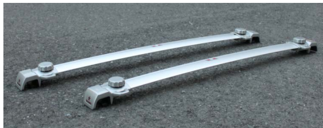
Roof cross bars aluminum brackets + aluminum bars
