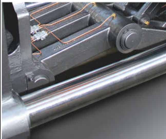
Wear resistant hard chromium plated tie bar is featured with high-tensile and high strength.
