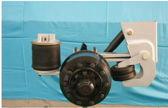
German type air suspension with lifting
