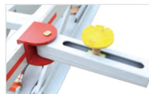
Four adjustable arms can wave in 180°range. They can lift nearly all kinds of car
