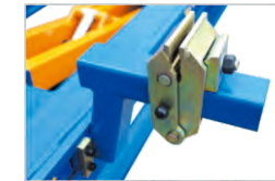
Main clamp jaw with patient can fix auto body, main clamp and cross-beam together with one screw.
