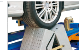
Multi-functional ramps also can be used as wheel support.
