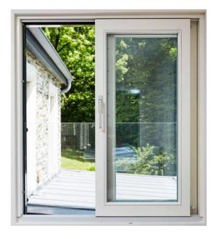
In this kind of door, the lift and slide panels use their own weight to compress the seals thus creating a completely weather-tight wall system when in the "down" position. When in the "up" position, it's operated like a normal sliding door, the panels are moved smoothly with a few pounds of pressure.
