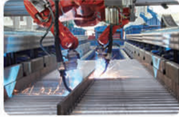
Shandong Huaxing Corrugated Web Beam Production line The first manufacture in China
