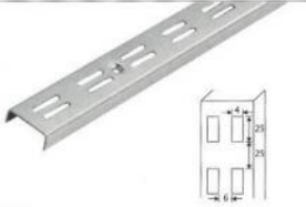
A002 产品名称 (Name): 长方双孔柱 15x20x15, 15x25x15, 17x30x17, 11x33x11, 13x33x13mm Rectangular double-hole column 15x20x15, 15x25x15, 17x30x17, 11x33x11, 13x33x13mm 厚度 (Thickness): 1.2mm, 1.5mm, 1.8mm, 2.0mm 规格 (Size): 1.5M, 1.8M, 2M, 2.4M
