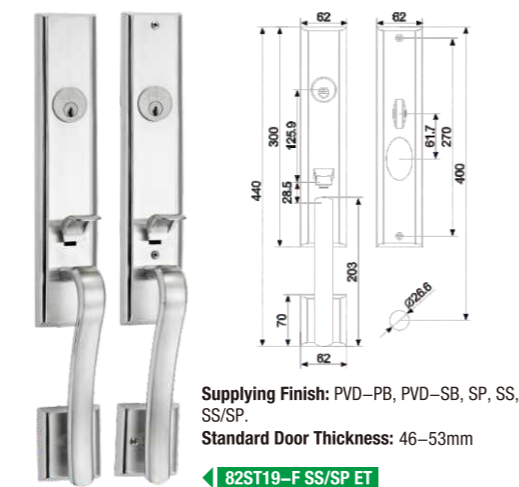
MODEL NO. : 82ST19 MATERIAL: Stamping stainless steel 304
