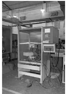
CNC For Keyway Milling Of Angle-cut-pin
