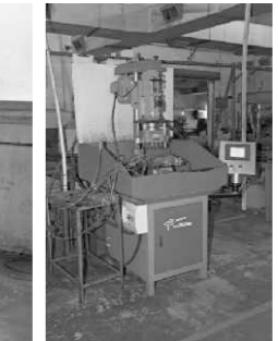
CNC For Pin Hole Drilling Of Cylinder Plug And Casing
