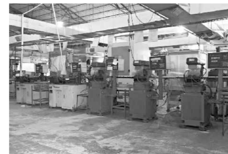
CNC For Keyway Milling Of Double-row-pin And Single-row-pin
