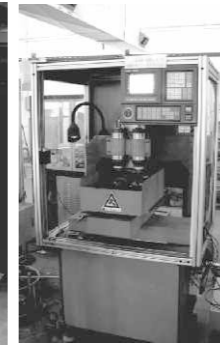
CNC For Pin Hole Drilling Of Cylinder Casing
