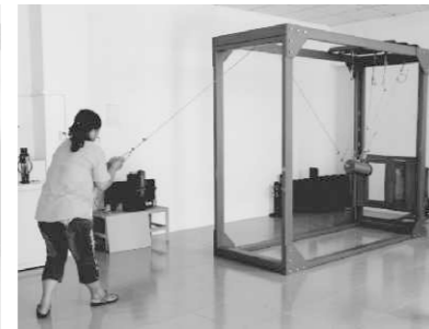
Horizontal Impact Test
