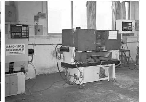
CNC For Plug Hole Drilling Of Cylinder Casing
