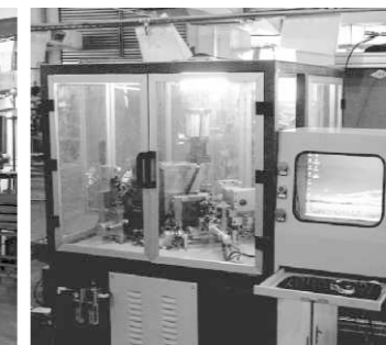
CNC For Keyway Milling Of Yale, Kwikset, Schlage and Weiser
