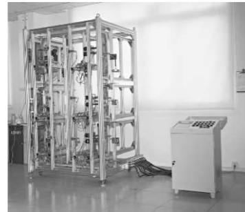
Multiple Cycle Test For Complete Set (Max. test 16 sets at the same time)
