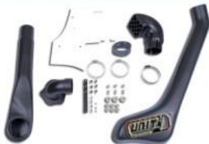
Nissan-Y61C SS17HF 9/04 onwards TD42-TI/ZD30DDT 4.2Litre-I6 /3.0Litre-I4 Material:LLDPE
