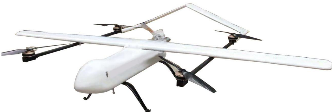
Fig.1 CL-3 Hybrid power Composite wing VTOL UAV
