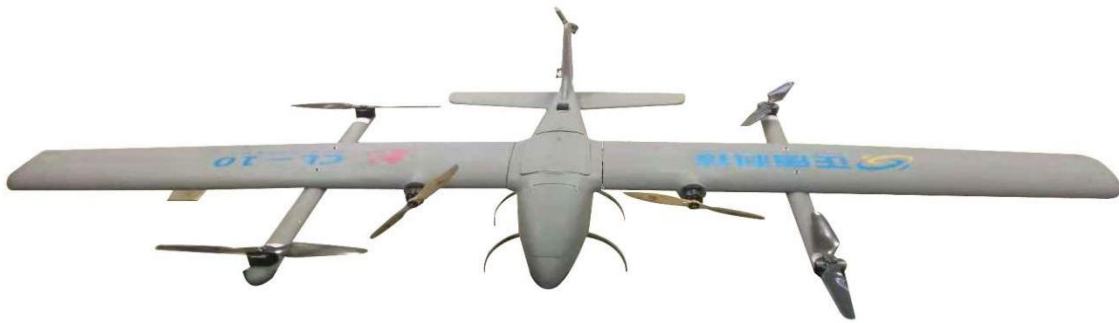
Fig.3 CL-10 Electrical composite wing VTOL UAV
