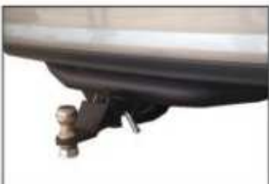
PW018736 REAR HITCH WITH RECEIVER & BALL WITHSTAND THE TENSION OF 6000LBS
